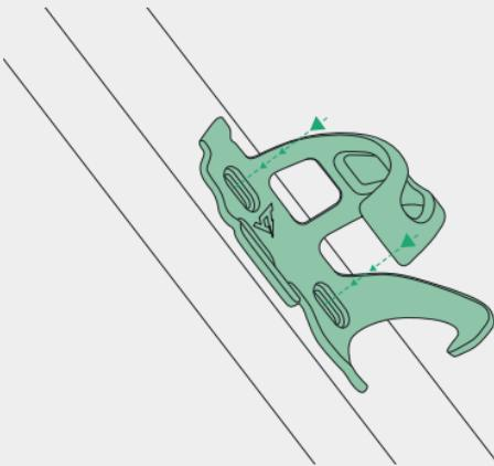
**1.2** Position the bottle holder over the threaded holes in the frame.
