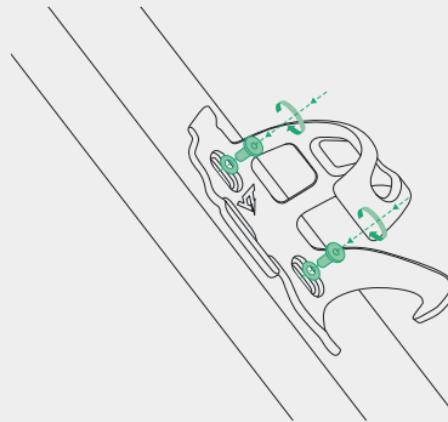
**1.3** Place the bolts and tighten them in the clockwise direction with a 3 mm Allen key (2Nm). Be sure to always use the washers.
